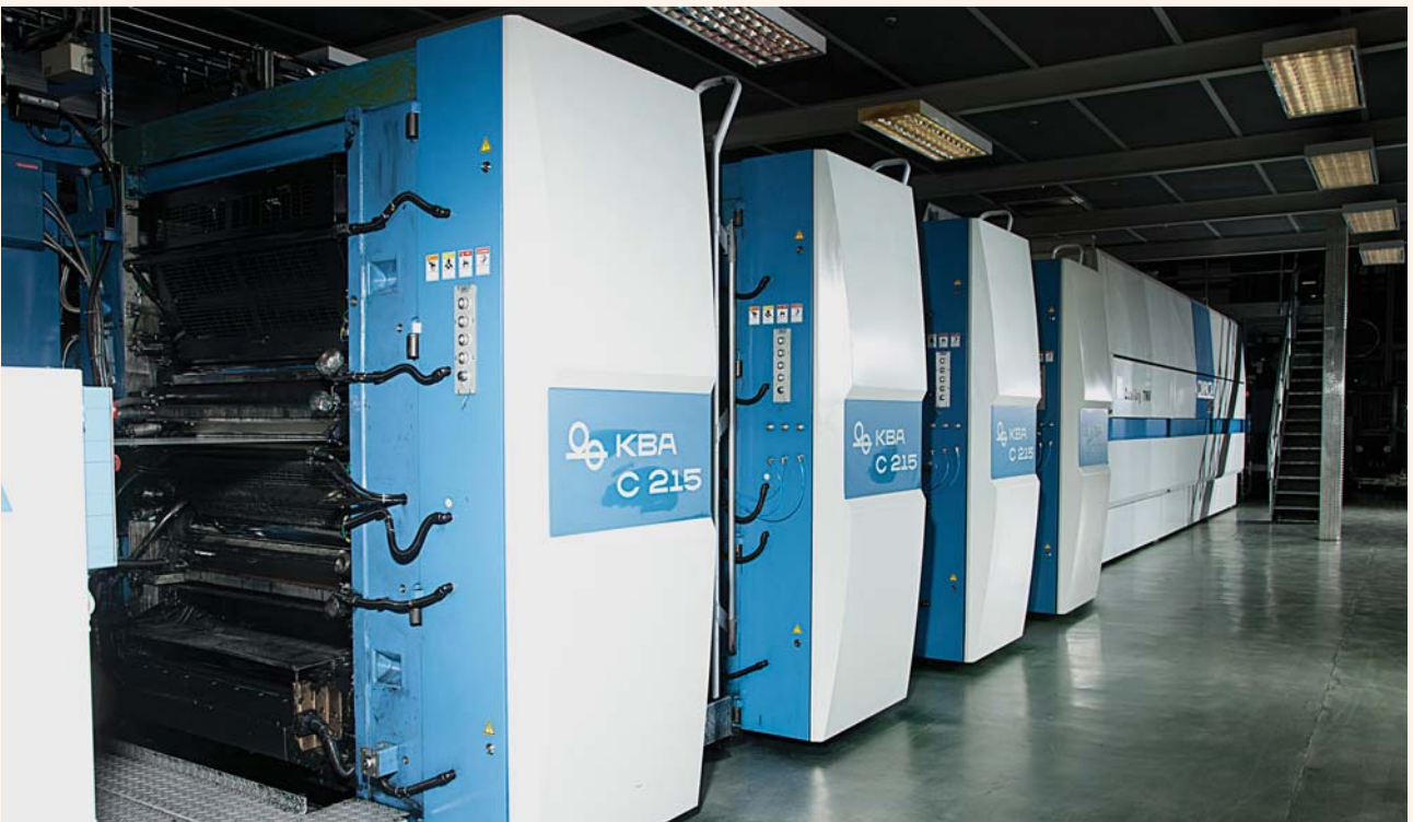
The new KBA C 215 16-page press installed at CTP Printers in Johannesburg
